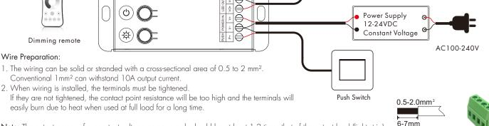
Note: The output power of a constant voltage power supply should be at least 1.2 times that of the output load (light strip), otherwise the full power output of the load can easily cause automatic flickering or shaking of the light.
